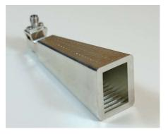
lightness. Indeed, this antenna is lighter than a machining one due to the realization by a 3D printer.
